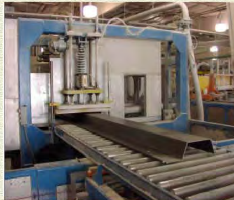
Step 5: Profiles' cutting of determined length
