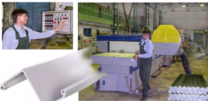
Manufacturing of composite profiles in the shopfloor of the enterprise by using pultrusion machine
