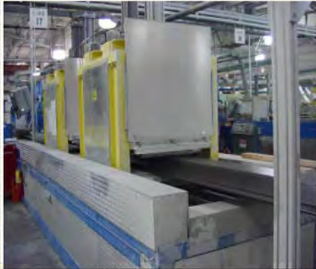
Step 4: Displacement of the profiles by using pulling machine
