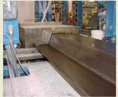
Step 3: Molding of profile in a die
