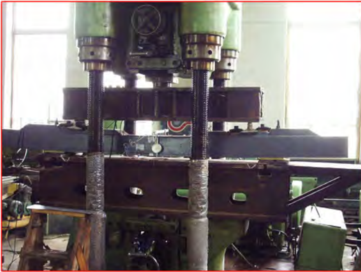
Testing phase of the assembled composite sleepers lattice on the simulated metal bridge span.
