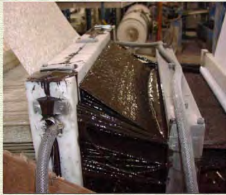
Step 2: Impregnation of glass-filler with resin
