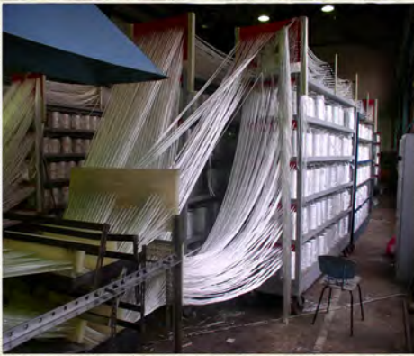
Step 1: Loading of glass-fillers into the die
