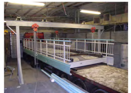
Loading of the finished bridge span in the workshop of the enterprise
